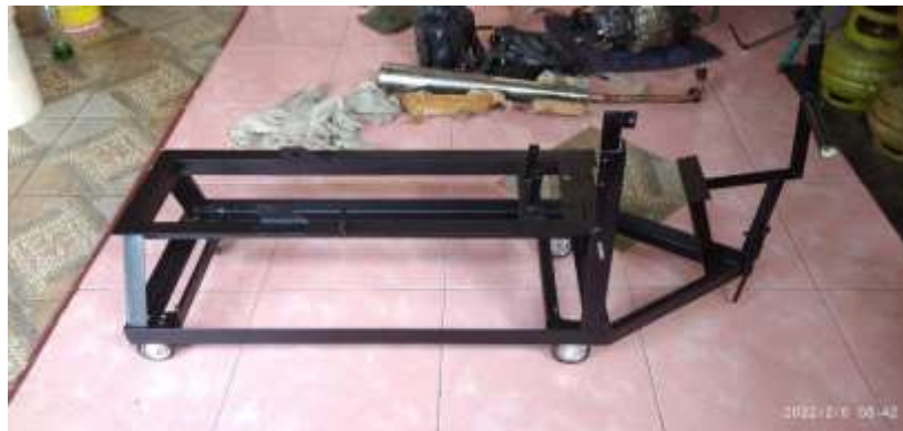
Gambar 4. 24 Chassis Alat Uji Rem Cakram Sepeda Motor
