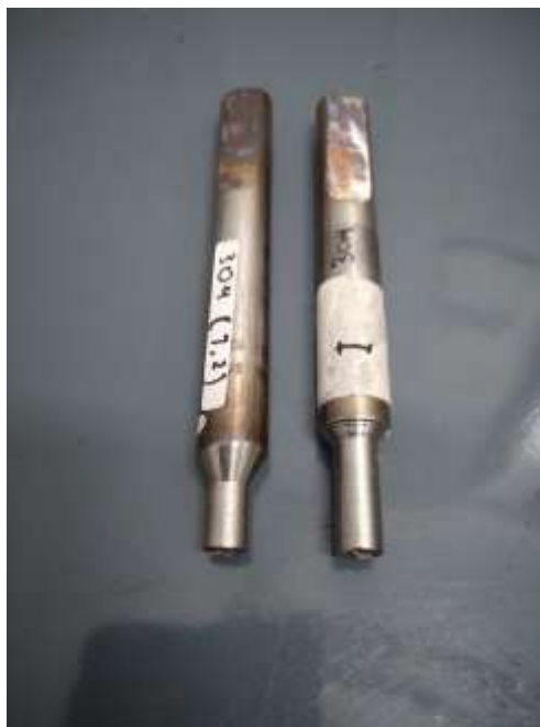
Gambar 4. 8 Hasil Uji Tarik Sampel 1
