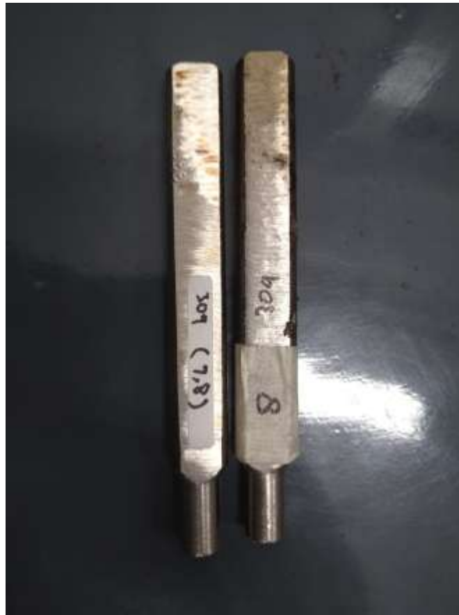
Gambar 4. 15 Hasil Uji Tarik Sampel 8
