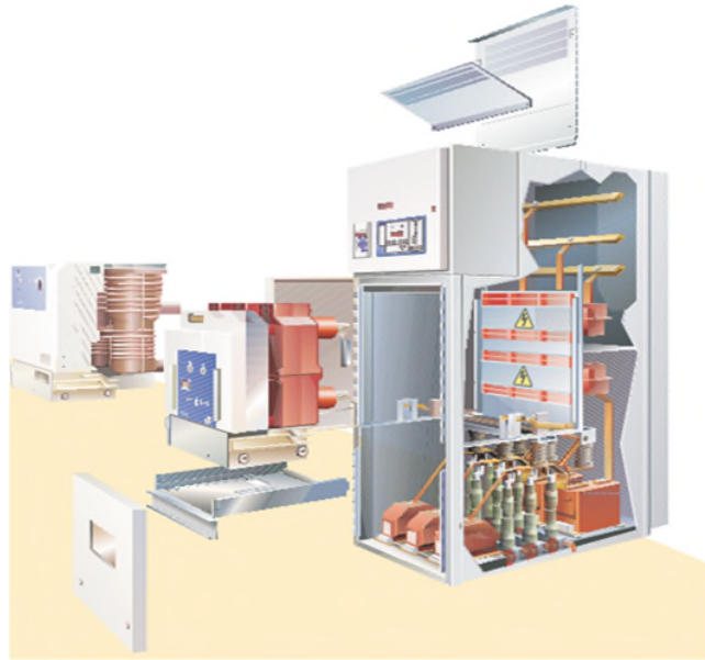
Gambar 2.6. Gambar Panel Distribusi 24kV Jenis Metal Clad (Gill, A.S, 1982).
